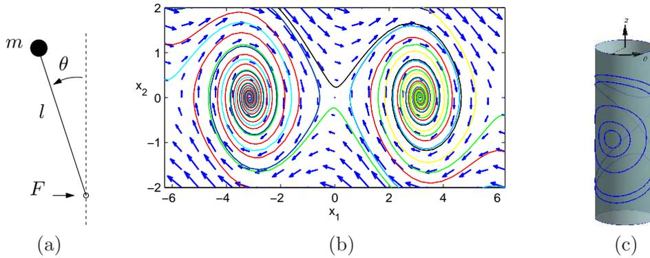
Figure 4.11: Phase portrait for a damped inverted pendulum: (a) diagram of the inverted pendulum system; (b) phase portrait with  $\theta \in [2\pi, 2\pi]$ ; (c) phase portrait with  $\theta$  periodic.
