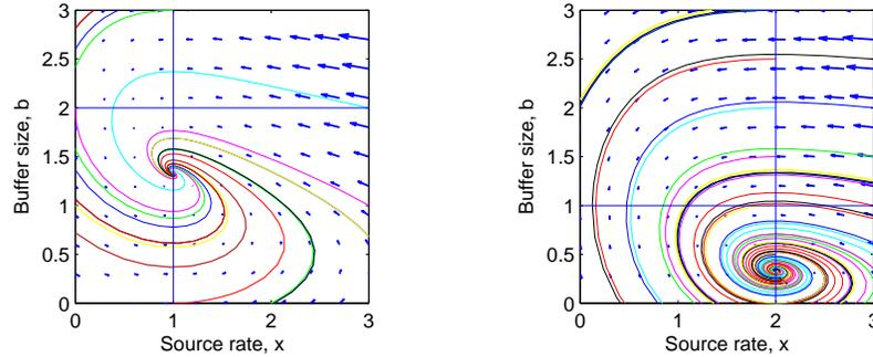
Figure 4.12: Phase portraits for a congestion control protocol running with a single source computer: (a) with router buffer size  $b_{\max} = 2$  Mb and link capacity  $c = 1$  Mb/sec and (b) router buffer size  $b_{\max} = 1$  Mb and link capacity  $c = 2$  Mb/sec.
