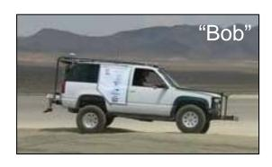
$$m\dot{v} = -bv + f_{\text{engine}} + f_{\text{hill}}$$
