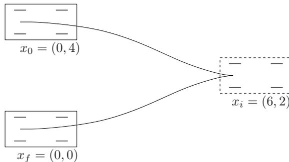
Your solution should consist of two segments: a curve from  $x_0$  to  $x_i$  with  $v > 0$  and a curve from  $x_i$  to  $x_f$  with  $v < 0$ . For the trajectory that you determine, plot the trajectory in the plane ( $x$  versus  $y$ ) and also the inputs  $v$  and  $\phi$  as a function of time.
