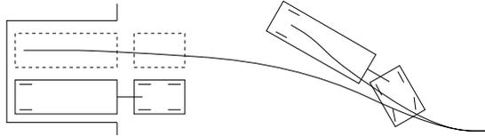
$$\begin{aligned}\dot{x} &= \cos \theta u_1 \\ \dot{y} &= \sin \theta u_1 \\ \dot{\phi} &= u_2 \\ \dot{\theta} &= \frac{1}{l} \tan \phi u_1 \\ \dot{\theta}_1 &= \frac{1}{d} \cos(\theta - \theta_1) \sin(\theta - \theta_1) u_1,\end{aligned}$$
