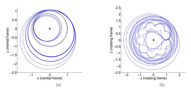
Figure 9: (a) Trajectory in the Saturn-Titan CR3BP which utilizes resonant gravity assists with Titan in order to iteratively reduce the orbit's semimajor axis. Over the course of its 23-month flight, the trajectory requires a surprisingly small total  $\Delta V$ : a mere 15 m/s. The central black disc denotes Saturn, and the thin black circle traces Titan's orbit. (b) The same trajectory, plotted in a rotating frame with Saturn and Titan fixed on the x-axis.
