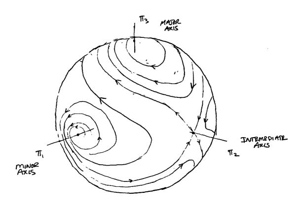
Figure 5: Angular Momentum Sphere Trajectories
