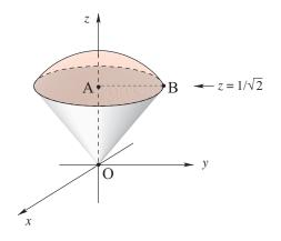
Notice that the triangle AOB has two sides of length  $1/\sqrt{2}$ , and hypotenuse of length 1, so the vertex angle AOB is  $\pi/4$ . Using this geometry and spherical coordinates, we find that a parametrization is
