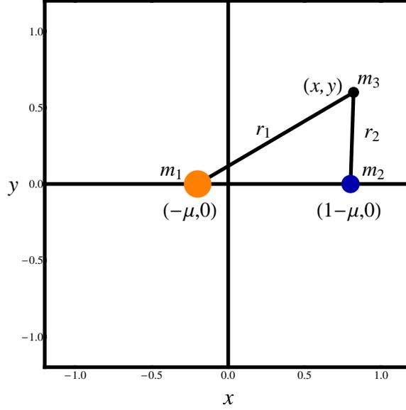
Figure 1: Rotating coordinate system in the circular restricted three-body problem. All units are nondimensionalized. The coordinate frame rotates counterclockwise with unit angular frequency so that the primary masses  $m_1$  and  $m_2$  remain fixed at the positions  $(-\mu, 0)$  and  $(1 - \mu, 0)$ , respectively.
