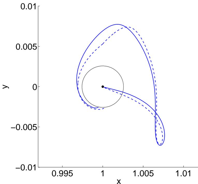
Figure 6: Locally optimal Earth-to-Moon trajectory (solid blue line) juxtaposed with the patched initial guess (dashed blue line) of Fig. 5. The central black disc denotes the Earth, while the thin black circle traces the Moon’s orbit. A  $\Delta V$  of 17 m/s is required for the optimal trajectory, a significant improvement over the patched trajectory’s  $\Delta V$  of 163 m/s.
