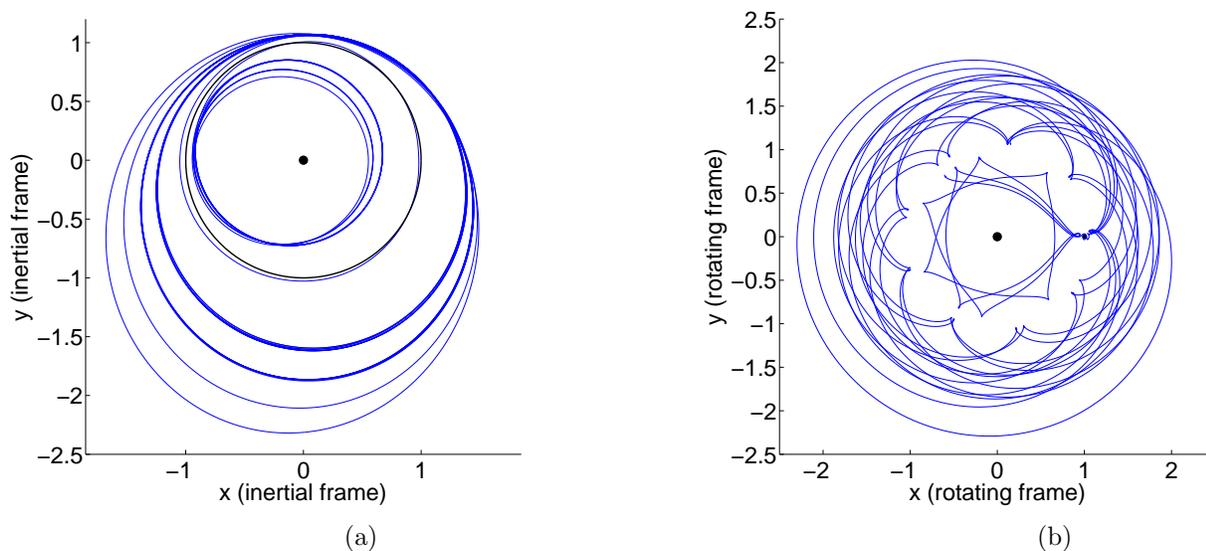
Figure 9: (a) Trajectory in the Saturn-Titan CR3BP which utilizes resonant gravity assists with Titan in order to iteratively reduce the orbit's semimajor axis. Over the course of its 23-month flight, the trajectory requires a surprisingly small total  $\Delta V$ : a mere 15 m/s. The central black disc denotes Saturn, and the thin black circle traces Titan's orbit. (b) The same trajectory, plotted in a rotating frame with Saturn and Titan fixed on the  $x$ -axis.
