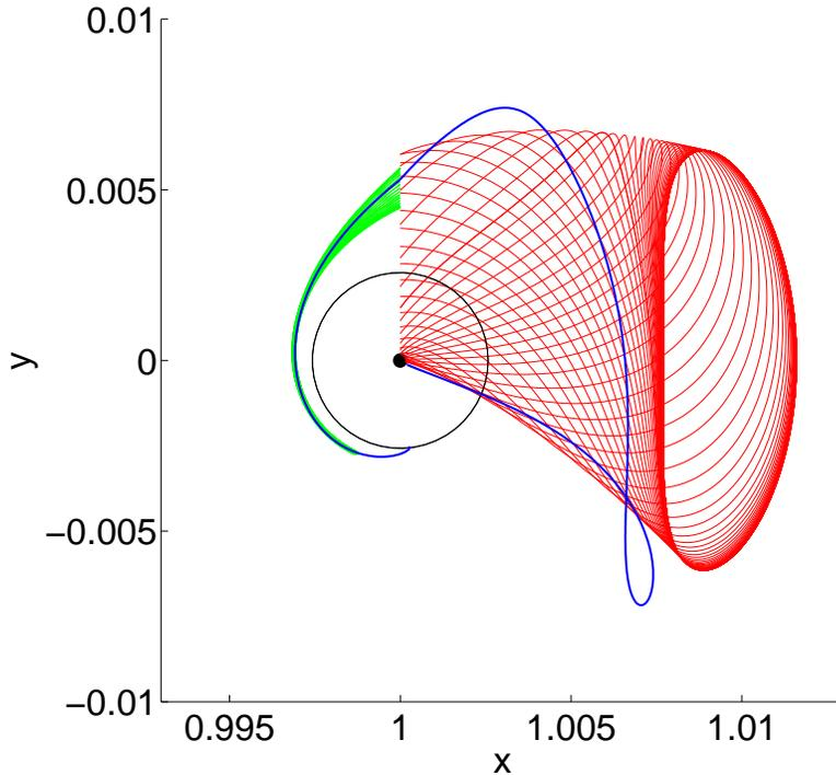
Figure 5: A patched Earth-to-Moon trajectory juxtaposed with the Sun-Earth (red) and Earth-Moon (green) invariant manifolds, in Sun-Earth rotating coordinates. The central black disc denotes the Earth, while the thin black circle traces the Moon’s orbit. A  $\Delta V$  of 163 m/s is required at the patch point.
