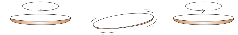
Figure 6.2: Rattleback Top . Sketch of the rattleback top initially spinning in the unstable direction, rocking back and forth, and then spinning in the opposite direction.
