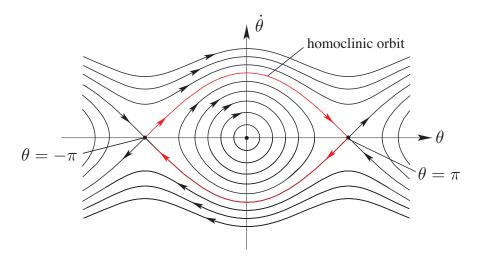
FIGURE 1.6.4. Phase portrait of the simple pendulum.
