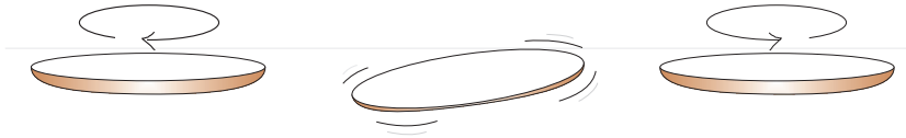
Fig. 6.1 Rattleback top. Sketch of the rattleback top initially spinning in the unstable direction, rocking back and forth, and then spinning in the opposite direction.
