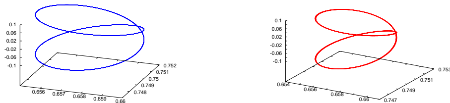
FIGURE 7. Spacecraft orbits suitable for binary observations. Left: Periodic orbit for the autonomous case. Right: 2D torus for the time-periodic case.
