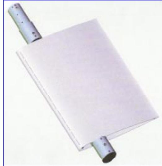
Figure 27. Drawing of 2D wind tunnel model blade section, showing DSJ slots.
