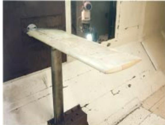
Figure 1. Full scale pitching 3D rotor blade model used for dynamic stall investigations (Ref. 8).
