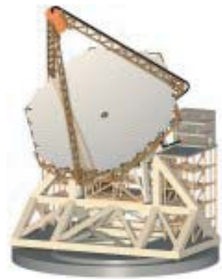
Figure 1. The GSMT f/1 telescope structure, with Cassegrain secondary and elevation axis behind the primary mirror.
