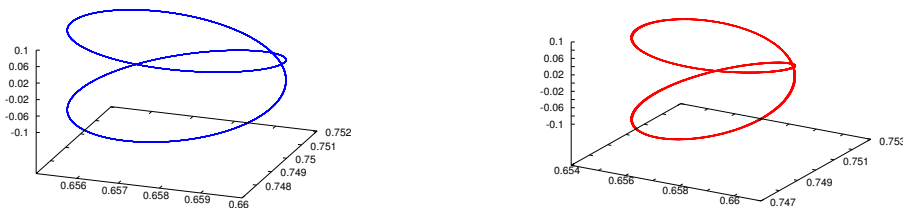
FIGURE 7. Examples of relatively high inclination orbits suitable for binary observations. Left: Periodic orbit for the autonomous case. Right: 2D invariant torus for the time-periodic case.
