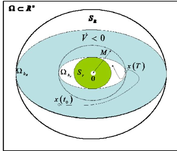
Figure 5.2: Representation of the sets  $S_r \subset \Omega_{b_r} \subset \Omega_{b_R} \subset S_R$  and the Ultimate Bound  $M$
