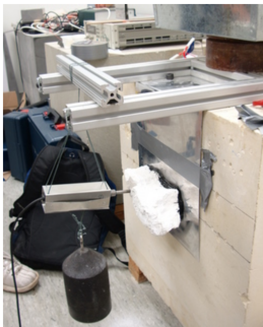
Figure 2: Experimental setup: the USDC is drilling into kaolinite
