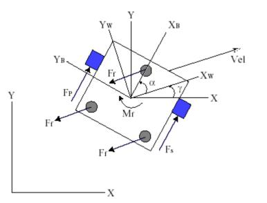
$$\begin{aligned} m\ddot{x} &= -\mu\dot{x} + (F_S + F_P)\cos(\theta) \\ m\ddot{y} &= -\mu\dot{y} + (F_S + F_P)\sin(\theta) \\ J\ddot{\theta} &= -\mu r_c^2\dot{\theta} + (F_S - F_P)r_f \end{aligned}$$
