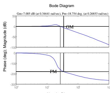
Bode Diagram. The top plot shows Magnitude (dB) versus Frequency (rad/sec). The bottom plot shows Phase (deg) versus Frequency (rad/sec). The gain margin (GM) is indicated as the frequency at which the phase crosses -180 degrees, and the phase margin (PM) is indicated as the phase margin at the gain crossover frequency.
