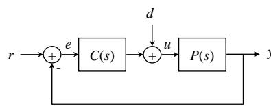
$$\begin{aligned} C(s) &= K_p + K_I \cdot \frac{1}{s} + K_D s \\ &= k \left( 1 + \frac{1}{T_I s} + T_D s \right) \\ &= \frac{k T_D}{T_I} \frac{(s + 1/T_I)(s + 1/T_D)}{s} \end{aligned}$$
