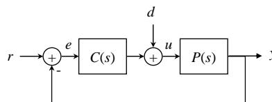
Block diagram of a feedback control system. The reference input  $r$  enters a summing junction with a positive sign. The error signal  $e$  enters the same summing junction with a negative sign. The output of this junction is the control signal  $u$ . This signal  $u$  enters a forward path block labeled  $P(s)$ . The output of  $P(s)$  is the system output  $y$ . A disturbance signal  $d$  also enters the summing junction with a negative sign.
