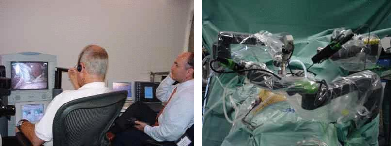
Figure 1.7 Remote robot surgery using the ZEUS system from Computer Motion Inc. The doctors on the left are in New York and the patient and the robots are in Strasbourg, France. Courtesy of Computer Motion Inc. Goleta
