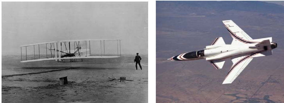
Figure 2.4. Flight systems: (a) 1903 Wright Flyer, (b) X-29 forward swept wing aircraft, in 1987. X-29 photograph courtesy of NASA Dryden Flight Research Center.
