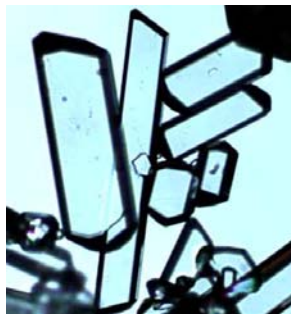
Figure 3.10. Microscope image of paracetamol crystals (paracetamol is the active ingredient in Tylenol), which shows the variability in crystal shape that can occur at a single time instance in a pharmaceutical crystallizer. Figure courtesy of Richard Braatz.
