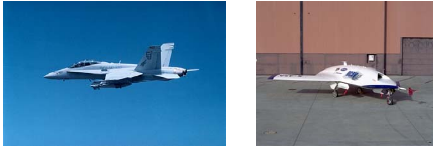
Figure 3.1. The F/A-18 aircraft, one of the first production military fighters to use “fly-by-wire” technology, and the X-45 (UCAV) unmanned aerial vehicle.
