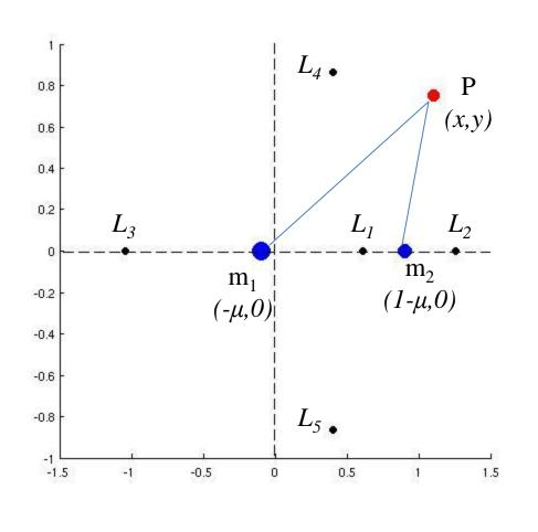
Equations of Motion for a test particle (spacecraft)  $\ddot{x} - 2\dot{y} = \frac{\partial\Omega}{\partial x}$  $\ddot{y} + 2\dot{x} = \frac{\partial\Omega}{\partial y}$  $\Omega = \frac{x^2 + y^2}{2} + \frac{1 - \mu}{\sqrt{(x + \mu)^2 + y^2}} + \frac{\mu}{\sqrt{(x - 1 + \mu)^2 + y^2}}$
